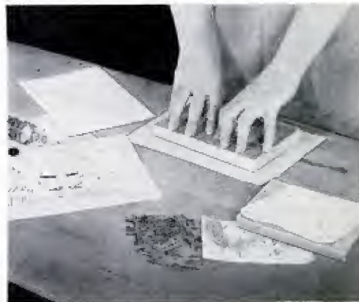
Above, using rubber cement, the finished printing plate is mounted on a wooden block. Below, after inking with linoleum-block ink, the printing block is used like a regular rubber stamp to reproduce the original design
